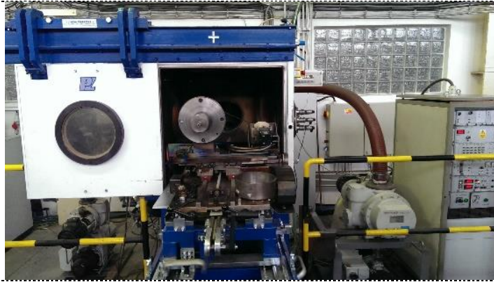
Figure 2. Universal electron beam welder PZ – EZ – ZH3.
